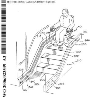
(57) Abstract: A system for assisting a person of limited mobility in moving from room to room within a home and performing essential activities includes a personal mobility device (40, 100, 1700, 1800, 2000) which includes transfer drivers (164) which engage a transfer system (210) to transition from a first elevation to a second elevation.
