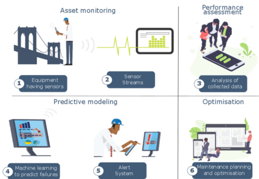
Figure 4.3. Building Intelligent Infrastructure for Resiliency and Maintenance
