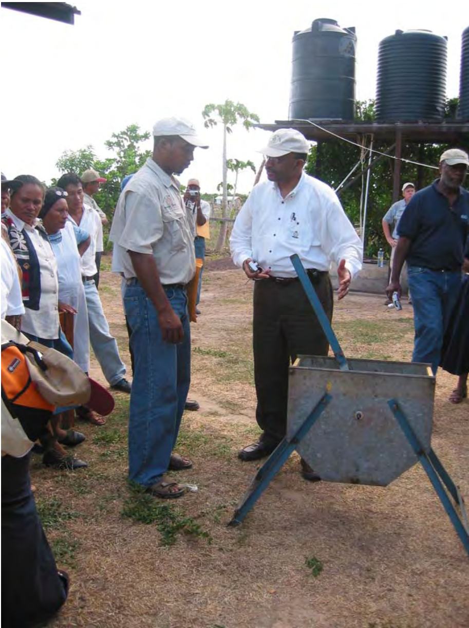
A simple peanut sheller used by small scale processors.
