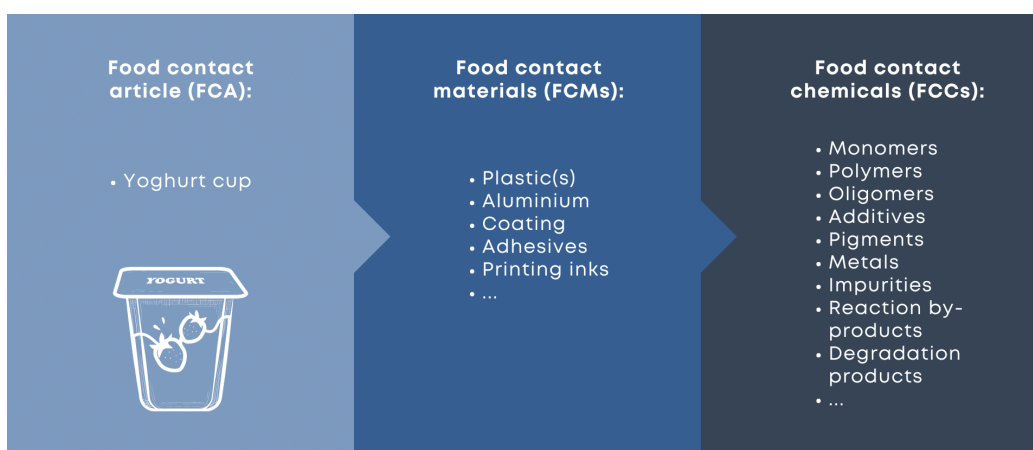
Figure 1. “Explanation of key terms. Food contact articles (FCAs) are combinations of different FCMs, which consist of food contact chemicals (FCCs) (e.g., a yoghurt cup made of polystyrene with printing inks and a coated aluminium cover glued on with adhesives). Food contact materials consist of mixtures of many FCCs. Food contact chemicals are defined as substances used and/or present in the manufacture of FCMs and/or present in FCMs and/or FCAs. Some FCCs are starting substances that no longer exist in the FCM/FCA. Some FCCs are generated during the manufacture of an FCM/FCA. Not all FCCs require an authorization, and they are not necessarily subject to risk assessment by an authority.” (adapted from [12]).
