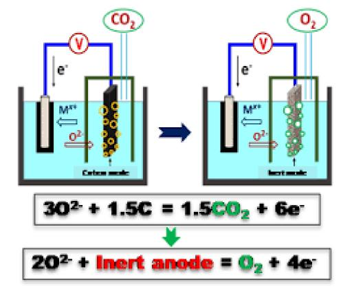
The chemical reaction of aluminum production in electrolyzers with inert anodes can be represented as follows:
