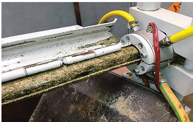
Bragdon fire log being formed in a mechanical press
