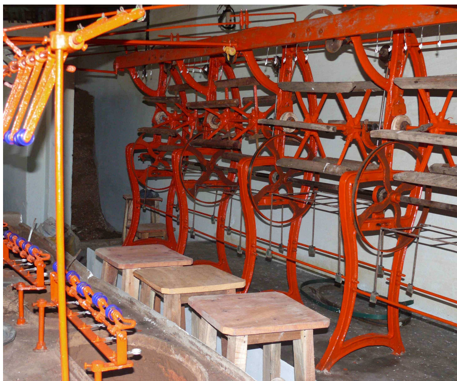
Picture 4: Motorised charkha for reeling, (see also Picture 6: Reeling), (Picture: Klaus Stocker)
