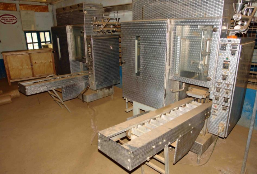
Figure A1 KDCS – Redundant milk packaging equipment provided by RDDP
